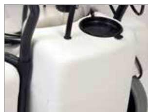
EXTERNAL DETERGENT TANK
